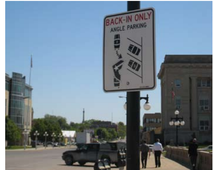
Back-in angle parking is safer for streets with parking and bike lanes
